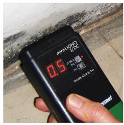
For building maintenance: The mini-Ligno S/DC is the right tool for checking mold stains to see how much moisture is still present in the wall.
