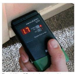
The mini-Ligno S/D meter shows true moisture percentages for drywall and wood. For other materials, comparative readings work best to determine high and low moisture levels.
