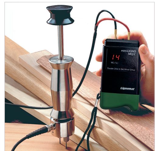
Adding depth electrode E12 with insulated pins allows measuring moisture up to 2" deep.
