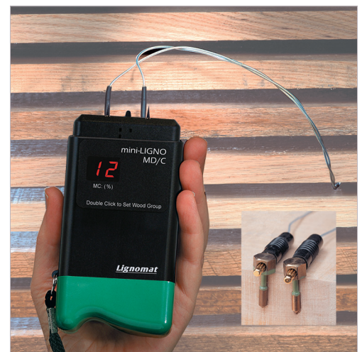
Adding probes and cables allows measuring moisture in the center of the stack without opening the hot kiln.
