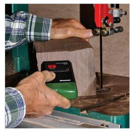
The mini-Ligno E/D is the meter for your next woodworking project to make sure the wood is dry enough. No more shrinking or warping.
